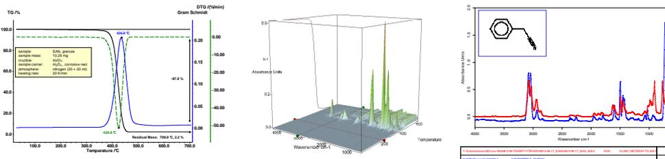
All measurements were carried out employing alumina crucibles, heating rate: 20 K/min, atmosphere: nitrogen, purge gas flow rate: 40 ml/min
